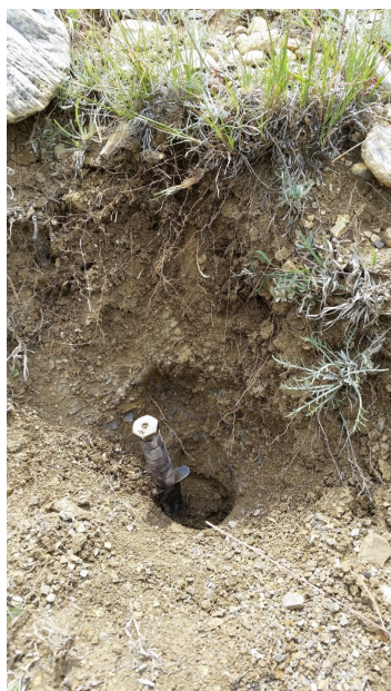
Figure 5. A typical Mion soil profile for the Slopes site. Note the gray shale fragments towards the bottom of the excavation, where developed soil grades into soft shale bedrock.
