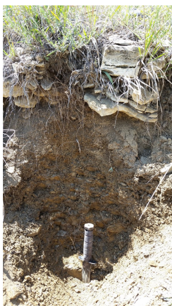
Figure 6. A typical soil profile for the Little component in the Slopes ecological site. Parent material is mostly derived from shale. Soft shale bedrock occurs at 27 inches (68 cm) in depth.
